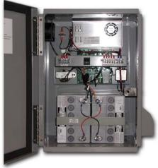
Plate 3. Interior view of an Outdoor-DC-UPS-8229 with output of 12 VDC, and 10 amperes maximum output.
