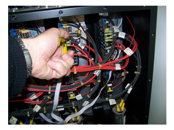
Remove fan connector from PCB header.
