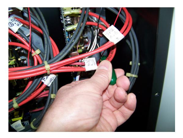
Remove the two (2) screws that fasten the PCB to the heatsink. Use angle phillips screw driver as space is limited. Save screws and washers.
