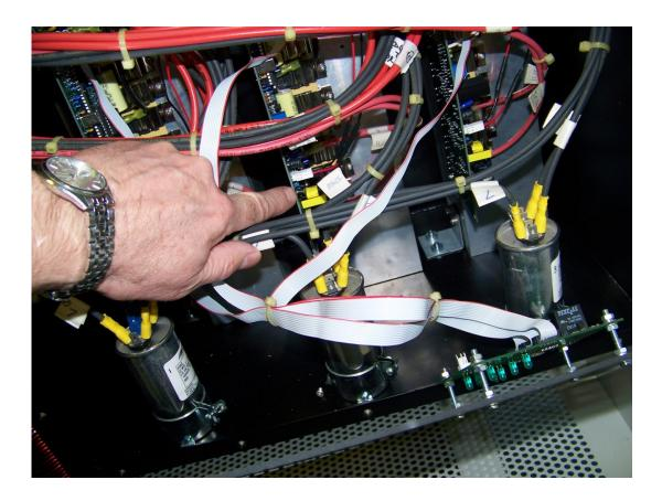
Remove 11 device clips using a phillips screw driver. Save screws and washers.
