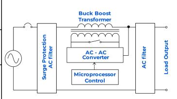
The high frequency Insulated Gate Bi-polar Transistor (IGBT) driven converter takes the incoming AC power, measures it against the nominal voltage reference and adds or subtracts voltage to achieve a precisely regulated output. The automatic bypass will be activated when there is a fault condition. Green LED is used to indicate Normal (regulating mode) operation.
