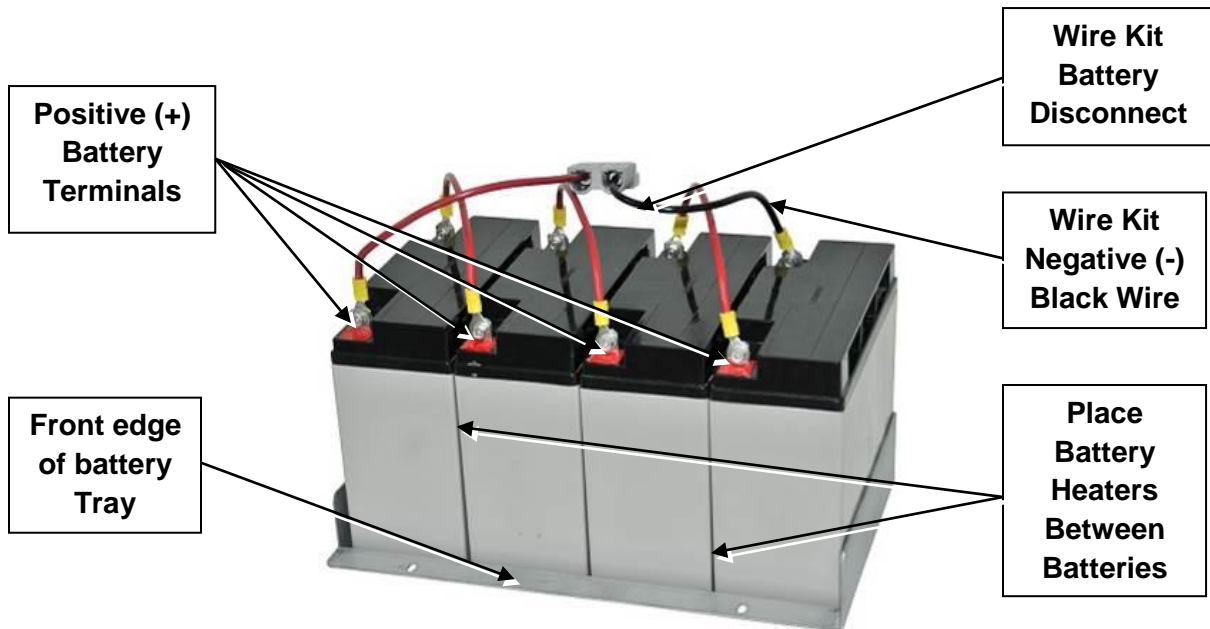
Figure 14: Four (4), NP 18-12 Battery Configuration Shown on removed Battery Tray
